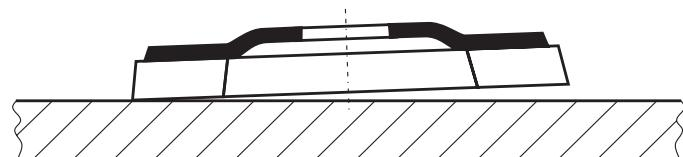
The flat shape is designed to grind edges and flat surfaces with a working angle of 0° to 15° degrees.
