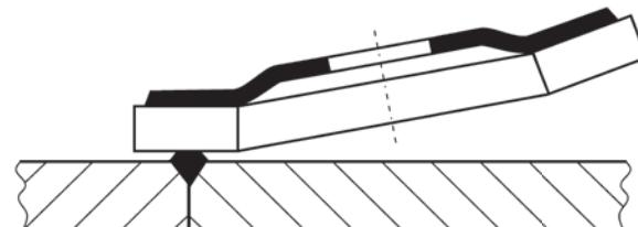
The angled shape is designed for spot grinding e.g. a weld seam with an ideal working angle of 15° to 25° degrees.
